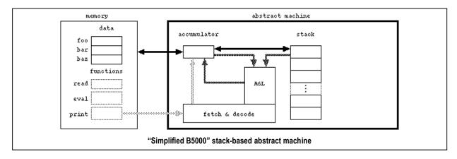
Literal values can be loaded into the accumulator. Values can be moved between the accumulator and the top of the stack, and moved between the accumulator and a named memory location. Operators use the accumulator as their first operand and take their other (if any) from the top of the stack. Results are left in the accumulator.
