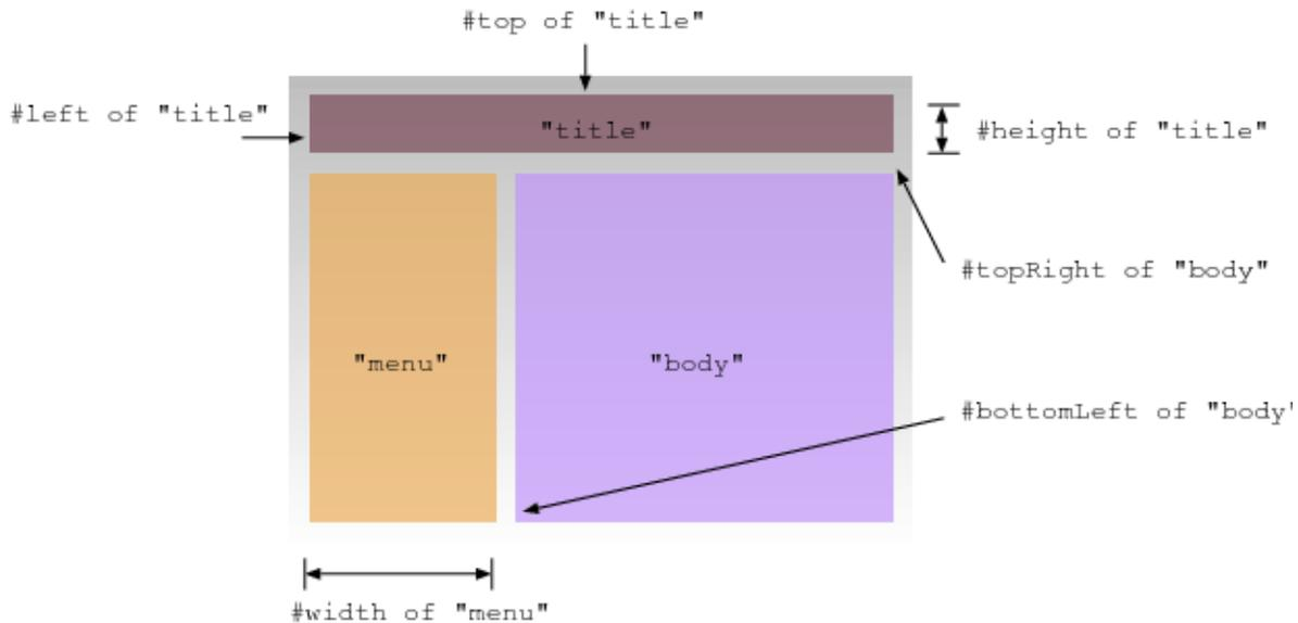
When layout is necessary, a `LSimpleLayout` recalculates each bounding box to satisfy all constraints. In the basic case, each constraint describes the subject box's attribute in terms of a reference box's attribute with distance parameters specified either in pixels (offset) or as a ratio (scale). Constraints are constructed by the `LSimpleLayout >> keep: method` family. The most generic form is `LSimpleLayout >> keep:of:to:of:scale:offset:.`
