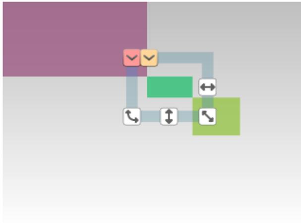
This layout arranges child boxes so that each box's bottom right corner touches next box's top left corner. You can download the complete source code from [LDiagonalLayout.st](#).
