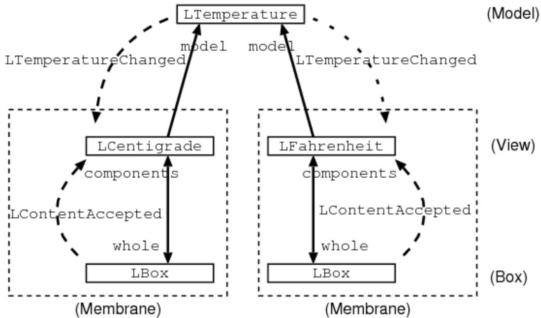
This diagram shows the relationships between the objects we need. It has three layers of object: model, view, and box. A solid line shows an explicit reference (an instance variable), and a dotted line shows an announcement. An **LTemperature** is a model which keeps the actual state: in this case, a temperature in Centigrade. **LCentigrade** and **LFahrenheit** are views of different perspectives of the model. Each view has its own **LBox**.
